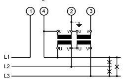
Current and voltage transformer connection
